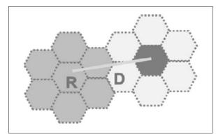
Total available frequency resources are divided into seven parts, each part consisting of a number of radio channels and allocated to a cell site. In a group of 7 cells, available frequency spectrum is consumed totally. The same seven sets of frequency can be used after certain distance.
